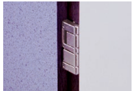
OBJECT HINGE (FA. PRAMETA) FOR COMPACT DOORS PANELS, DOOR THICKNESS 10 -13 MM. SINGLE AXIS PIVOT POINT.
