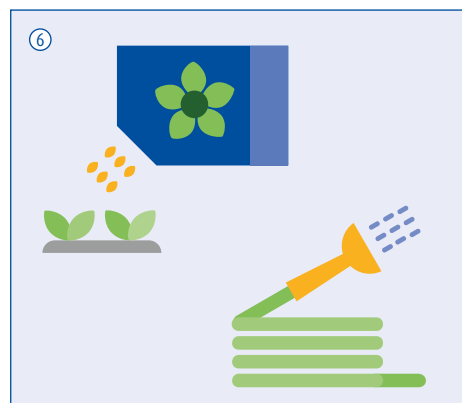
Fertilize the vegetation after the installation with the Urbanscape fertilizer and irrigate it copiously.
